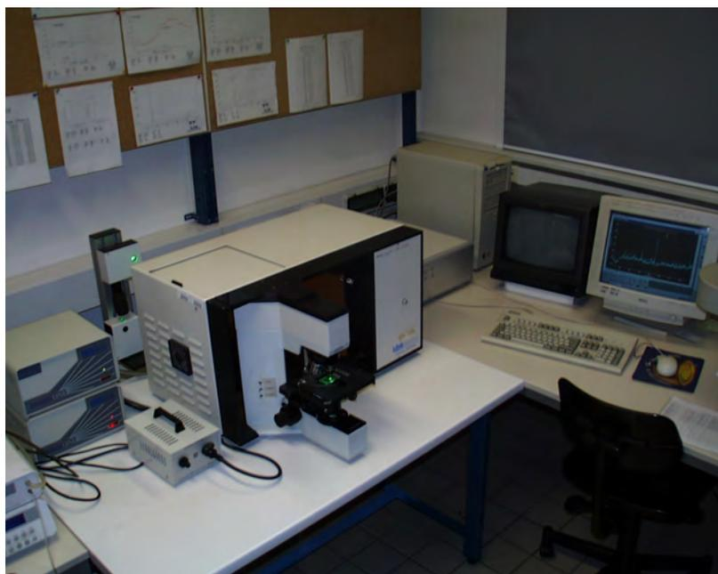
**Fig. 2.** The ISA Jobin Yvon LABRAM (Horiba) laser Raman microprobe, combined with an Olympus BX 40 microscope at the chair of Resource Mineralogy, Montan-University Leoben, Austria.
