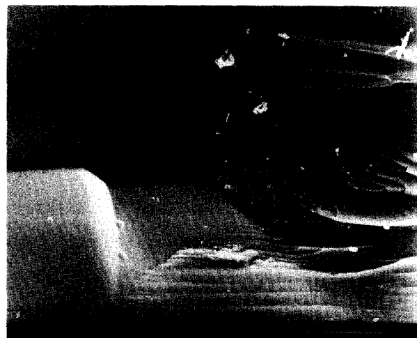
FIG. 6. SEM photomicrographs of crack surfaces, created by quenching the quartz core 2 in water after heat treatment at 623\ \text{K} before the original experiment E421. The morphology varies between smooth curved planes and a feather-like pattern of small steps.
