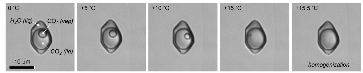
The homogenization temperature of +15.5 °C (in the liquid phase) corresponds to a density of 0.8168 g·cm-3. The microthermometer has an accuracy of 0.1<sup>°</sup> in this temperature range, and a precision of 0.1°C. Therefore, the uncertainty in density calculation is ± 0.001 g·cm<sup>-3</sup>
